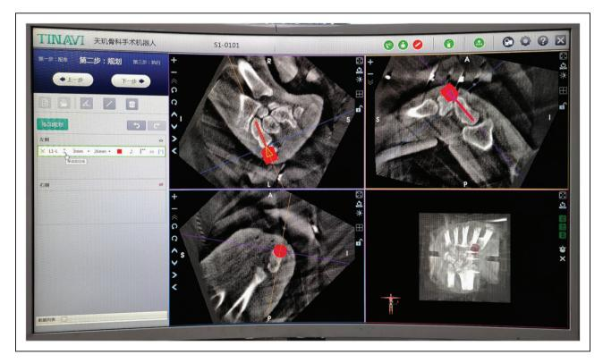
**Figure 3.** Graphical user interface of the surgical planning software in the TiRobot workstation. The surgeon can determine the optimal screw trajectory in the central zone of the scaphoid by modifying the screw path in the sagittal, axial and coronal planes.
