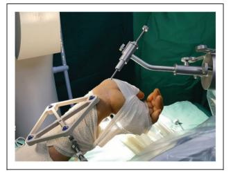
**Figure 4.** The surgical planning is communicated to the stereotactic robot arm, which automatically manoeuvres an effector gripper attached to a K-wire aiming guide to the planned trajectory.
