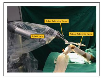
**Figure 1.** The wrist is extended and securely affixed to a wrist positioning jig. The patient reference frame is fixed onto the positioning jig. The robot reference frame is attached to the robotic arm.
